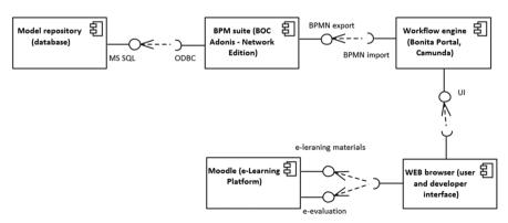
Figure 4. Components diagram of BPM laboratory
