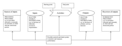
Fig. 1. A schematic representation of a single process
