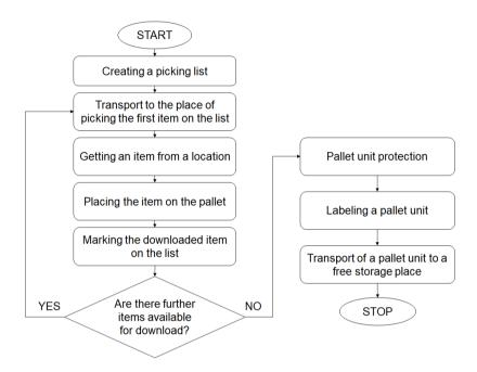
Figure 9. The picking process after the change
