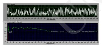
Fig. 3. The charts of the VoIP traffic with a small load and the Hurst exponent value obtained using the absolute value method.
