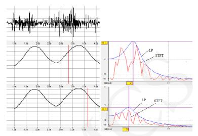
Figure 4 Comparison of the location and the maximum amplitude of the spectrum in the time window at the end of contraction and the beginning of extraction of the biceps muscle of a woman. From the top left: the waveform and two windows on goniometer chart, on the right appropriate STFT (red lines) and LP (blue lines) spectrum
