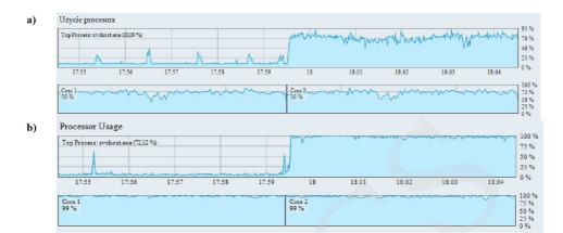
Fig. 11. The CPU usage for the VPN tunnel with SSTP/IPsec in FastEthernet: a) server; b) client.
