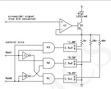
Fig. 1. Part of adapter controlling RED component
