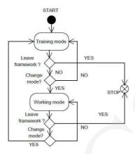
FIG. 4. Switching between Working and Training Modes
