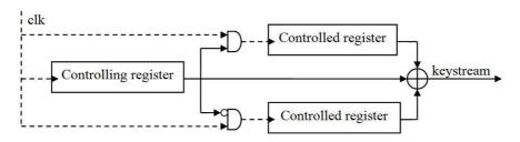
Rysunek 2. The Modified Alternating k-Generator
