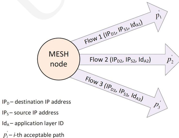
Fig. 9. Hashing Function – Load Balancing.
