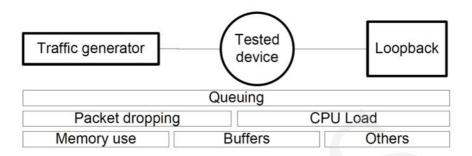
Fig. 1. Stress test – connection diagram.
