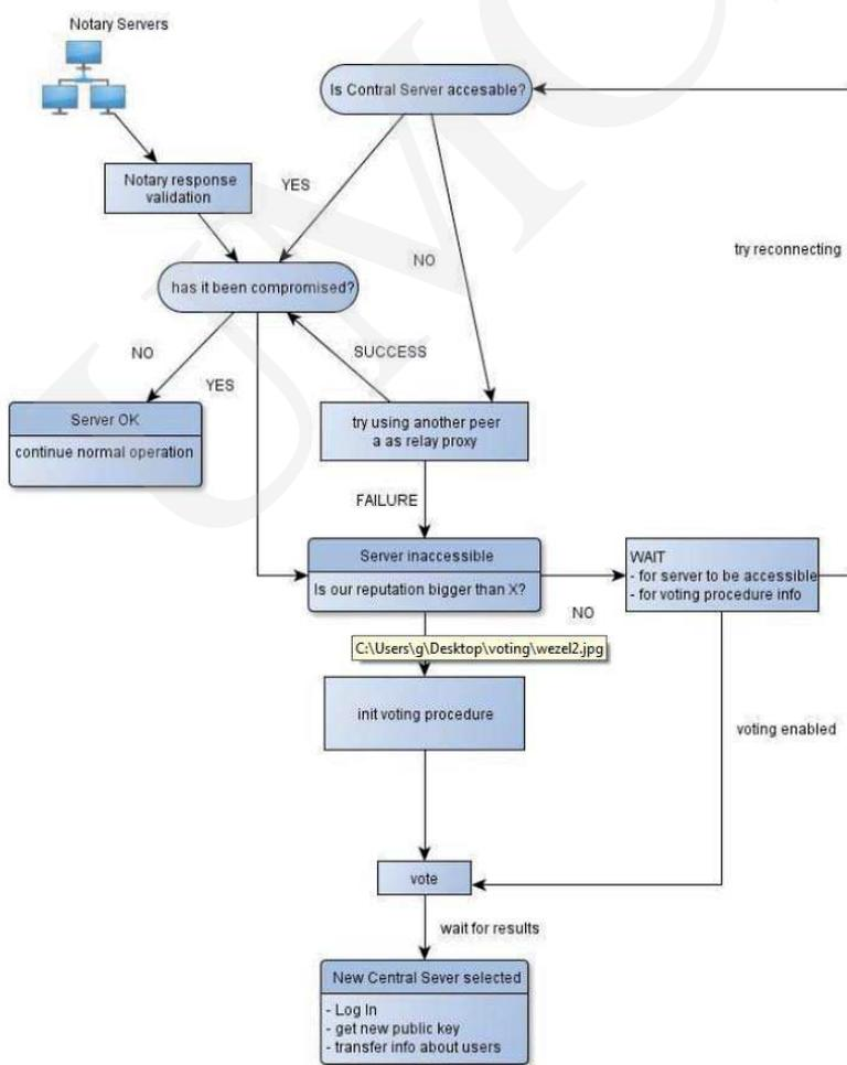
Fig. 1. Self-healing schema – from the peer side.
