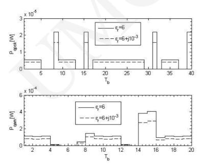
Fig. 5. Power of the QPSK (top) and 16QAM (bottom) signals as the function of the bit period for a lossless dielectric with  $\varepsilon_r = 6$  (continuous line) and in dielectric with  $\varepsilon_r = 6 + j 10^{-3}$  (dashed line) for which we considered propagation at r = 100m.
