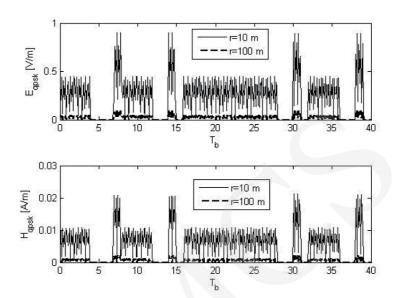
Fig. 3. Electric (top) and magnetic (bottom) fields for the QPSK modulated signal at r=10m (continuous line) and at r=100m (dashed line) when  $\theta=30^{\circ}$ .
