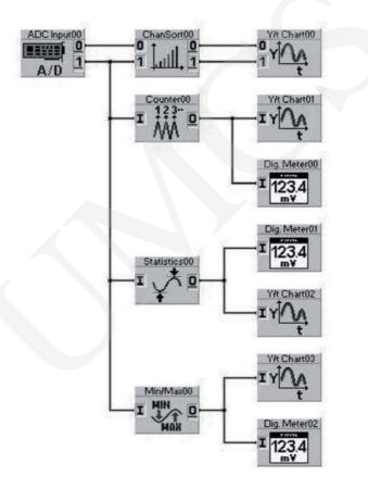
Fig. 1. Acquisition of signals from the inductive sensor and basic methods of their processing.
