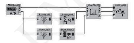
Fig. 3. Averaging and analysis of the maximal and minimal values of the measuring signal of the previously defined block of measuring data.
