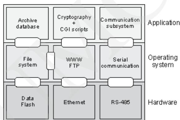
Fig. 3. Basic components of the server program.
