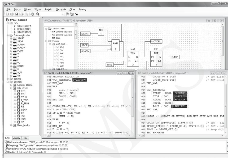
Fig. 5. Main window of CPDev programming environment.
