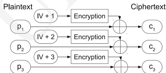
Fig. 8. Block cipher in the Counter (CTR) mode.
