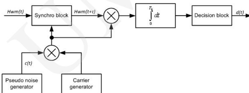
Fig. 6. Schematic diagram for the watermark extractor.
