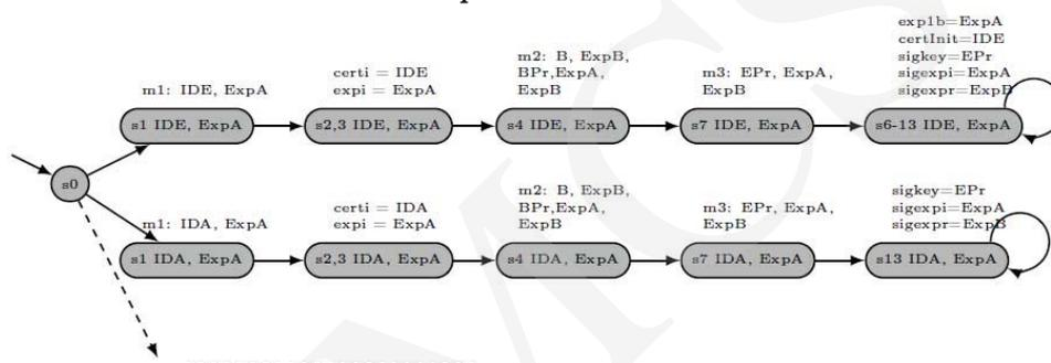
Fig. 3. Kripke structure constructed from automaton from Fig. 2.
