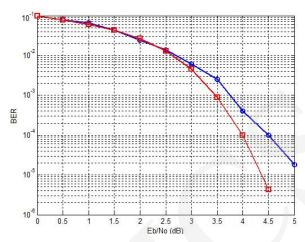
Fig. 3. Bit error rate for [16807, 4802] code (square) with  $a \in \{0, 1\}$  and chosen vertex [l] = [0, 0, 0, 0, 0] and [343, 98] code (circle) with  $x \in \{0, 1\}$  and chosen vertex (p) = (0, 0, 0, 0, 0), both based on AH(7, 7).
