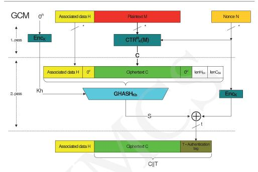
Fig. 6. GCM authenticated encryption scheme.
