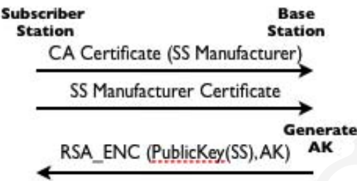
Fig. 4. Station Authentication Process.
