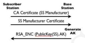
Fig. 4. Station Authentication Process.
