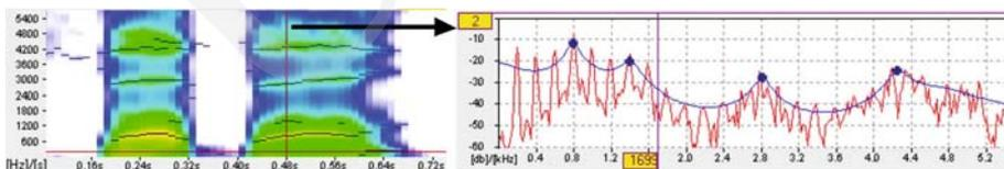
Fig. 4. Spectrogram (on the left) the utterance "papa" (sampling rate 22kHz) and the spectrum (spectrogram intersection) of the selection in the spectrogram computed with FFT and LP. The linear prediction order  $p=22$ .
