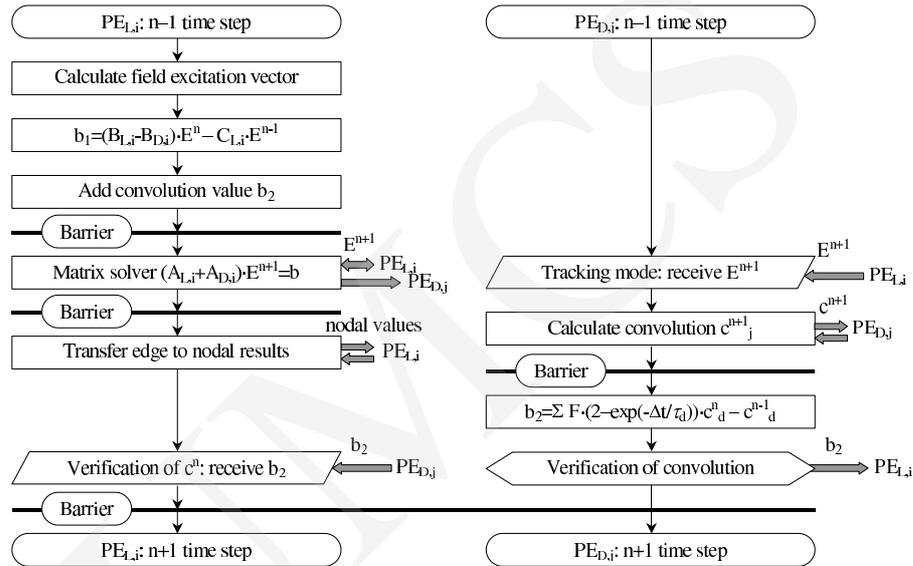
Fig. 4. Decomposition of computations among threads for a single time step
