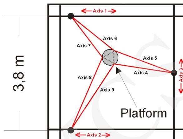
Fig. 3. The top view on the 9-DOF robot
