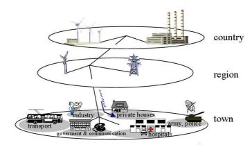
Fig. 1. Typical hierarchy of electric energy distribution system
