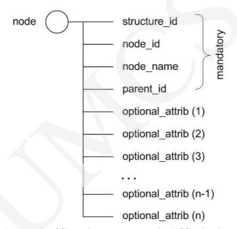
Fig. 2. The GS's node repository in the HCS's database
