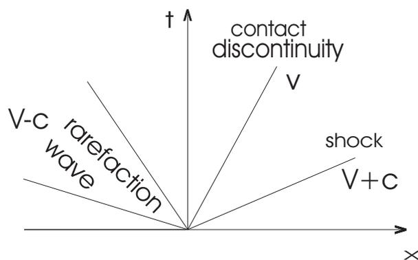
Fig. 1. Wave structure of the Riemann problem for the one-dimensional Euler equations
