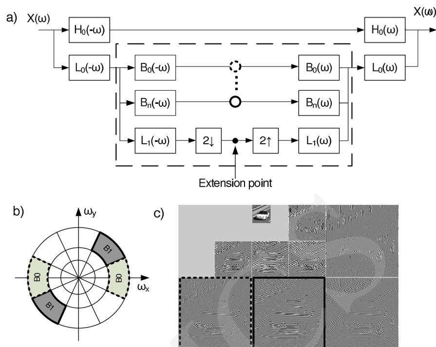
Fig. 1. Steerable pyramid transform: a) – the transformation filter structure, b) – the Fourier magnitude spectrum with marked frequencies passed by the filters  $B_0$  and  $B_1$ , c) – two levels of a sample image decomposition with four filtering directions
