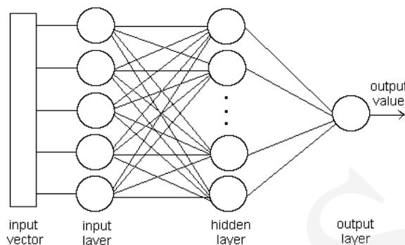
Fig. 2. The scheme of feed-forward network
