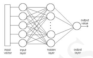
Fig. 2. The scheme of feed-forward network
