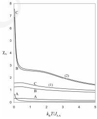
Fig. 5. Magnetic susceptibility  $\chi_X$  (X = A, B;  $\chi_C = \chi_A + \chi_B$ ) vs. reduced temperature  $k_B T/J_{AA}$  for diluted ( $x = c_C$ ) binary amorphous structure ( $A_p B_{1-p})_x C_{1-x}$  with  $z_A = z_B = 3$ , and two sets of parameters described above in the text
