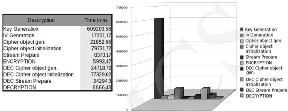
Fig. 7. Time consumption of the Blowfish algorithm
