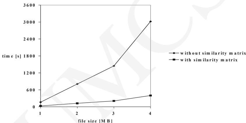
Fig. 5. Clustering time for two versions of algorithms
