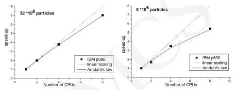
Fig. 2. Hard scaling properties of the parallel TRQR for two different numbers of pseudo-particles
