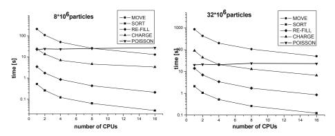
Fig. 3. Execution times for most important code pieces as a function of CPU number
