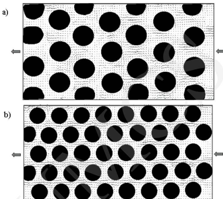
Fig. 5. Velocity vectors (ODP – PIV algorithm), a) Triangular – staggered arrangement d20t30TS for  $V_L = 0.69$  m/s and  $V_G = 0.69$  m/s, b) Triangular in-line arrangement d20t30QL for  $V_L = 0.67$  m/s and  $V_G = 0.67$  m/s
