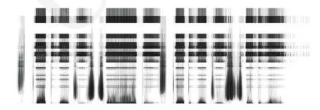
Fig. 10. Spectrum of 3-secunds speech signal with badly normalized scales. We can see stripes of overstated values (darker stripes) for scales with to large energy
