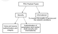
Fig. 2. Available PDU payload types
