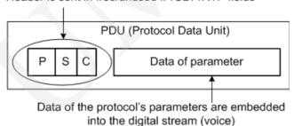
Fig. 1. General PDU characterization
