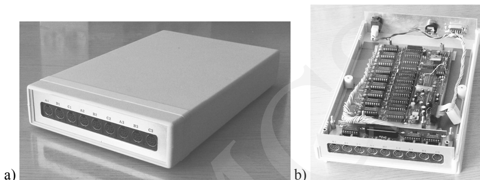
Photo 1. Recorder of curves I = f(U) : appearance of the recorder (a) and its interior (b)
