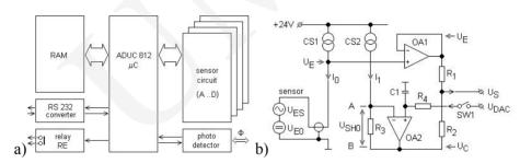
Fig. 2. Block diagram for the recorder (a) and single measurement channel (b)
