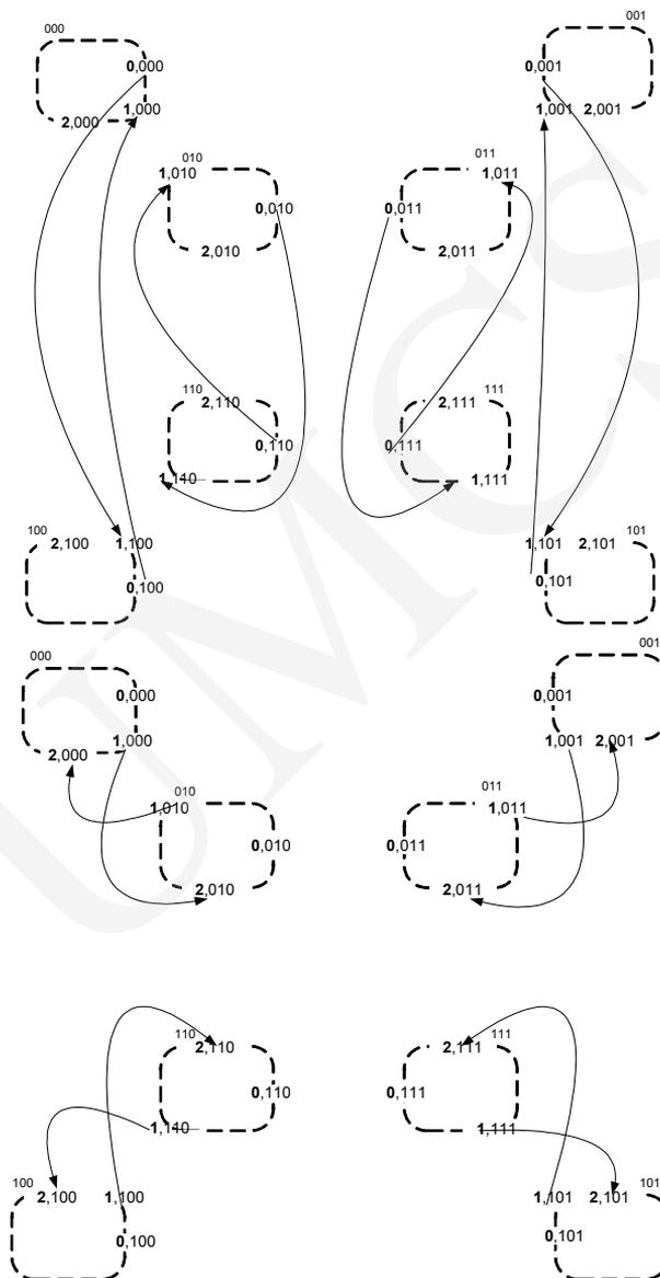
**Step 2.** We connect rings  $R_A$  and  $R_B$  using undirected edges which connect the node of ring  $R_A$  with the left part of address equal  $(K-1)$  to the node of ring  $R_B$  with the left part of address equal  $(0)$ . Using the previous denotation we can describe step 2 as connection between:  $(k-1, a_{k-1}a_{k-2} \dots a_i \dots a_1 a_0)$  and  $(0, a_{k-1}a_{k-2} \dots a_i \dots a_1 a_0)$ . For  $H(3,2)$  i  $R(3)$  we have:
