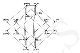
Fig. 1. Example of the product network of deBruijn(2) and hypercube (2)
