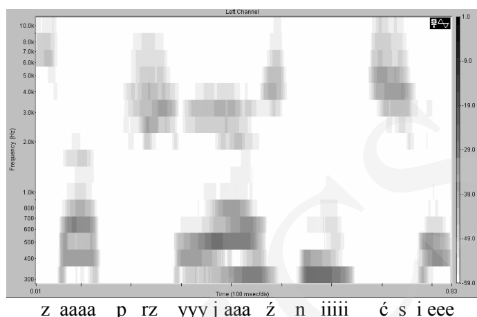
Fig. 1. Spectrogram of an utterance fragment „zaprzyjaźnić się” after FFT with the application of twenty one 1/3-octave bands and A-weighting filter
