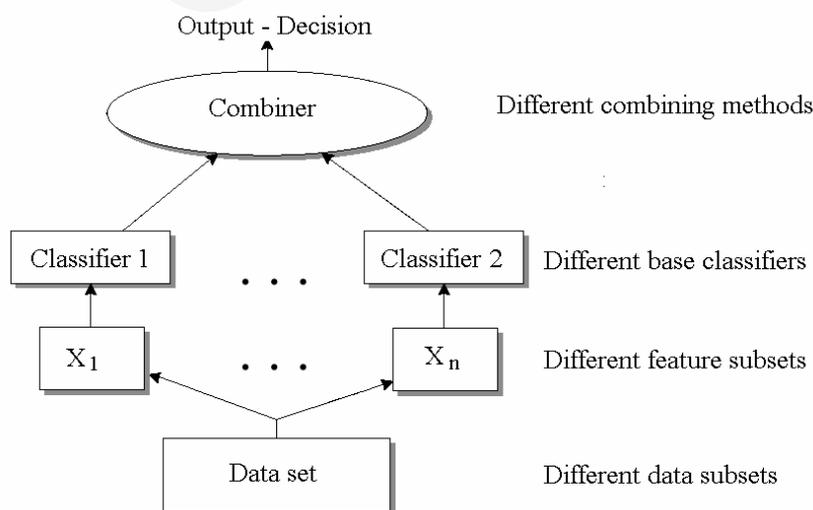
Fig. 1. The architecture of an ensemble system
