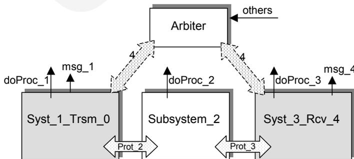
Fig. 4. Phase-2 structural model of the system
