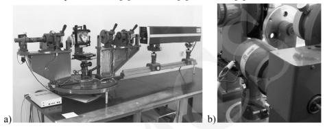
Photo 1. Ellipsometer EL11D: general view (a) and step motor with gearbox (b)
