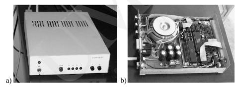
Photo 2. Controller of ellipsometer EL11D: general view (a) and interior (b)
