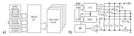
Fig. 1. Block Diagram for ellipsometer controller (a) and motors control system (b)
