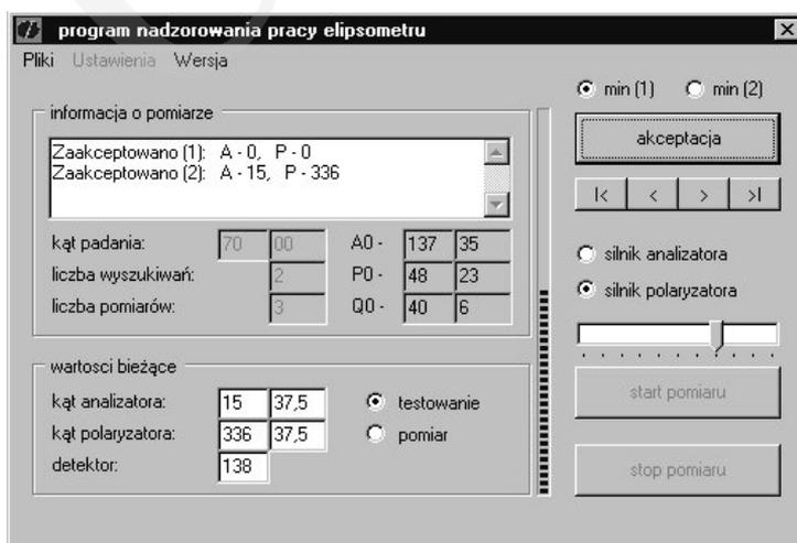
Fig. 4. Ellipsometer operation management program – graphical interface
