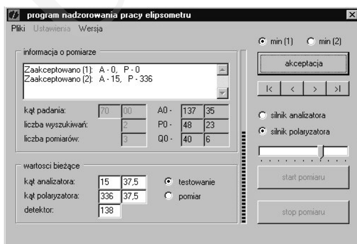
Fig. 4. Ellipsometer operation management program – graphical interface
