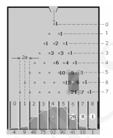
Fig. 1. A screenshot of the Flash movie frame [5] with a scheme of indexing layers and bins. The bolded figures denote the number of possible paths to the given rod (scatterer)
