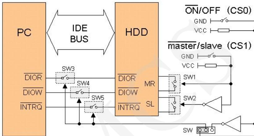
Fig. 3. Circuit scheme of the HDD switch
