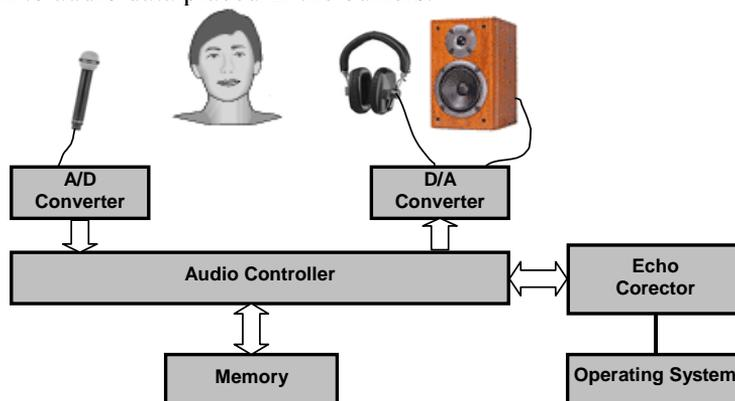
Fig. 2. The principle of speech echo-corrector operation
