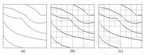
Fig. 4. Example of isobars and their decompositions on the third level: (a) original image; (b) beamlet decomposition; (c) bent beamlet decomposition
