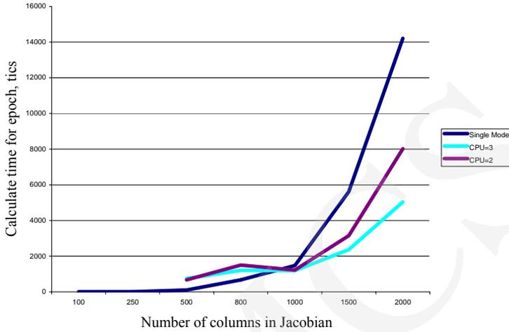
Fig. 2. Dependence of training time on the number of columns in Jacobian in single computer and 2,3 processor cluster
