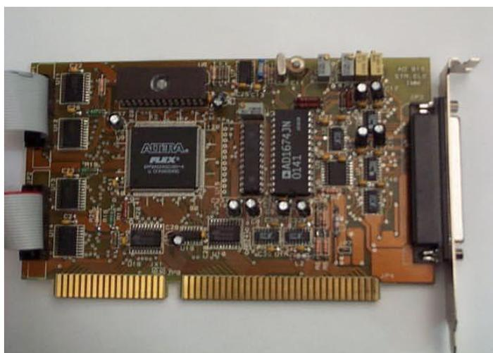
Fig. 3. The analog-digital card ADC615
