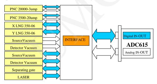
Fig. 4. A schematic diagram of spectrometer – card connections
