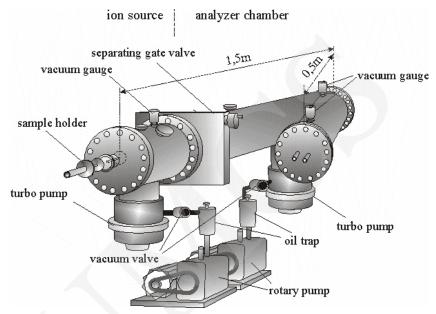
Fig. 2. The vacuum system of the TOF spectrometer
