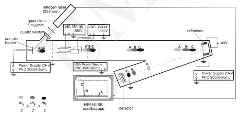
Fig. 1. An electrical TOF MS scheme and idea of ions formation and separation in this spectrometer
