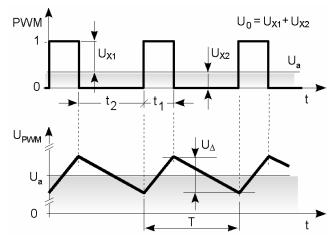
Fig.3. Saw-shape deformation of the analog PWM signal
