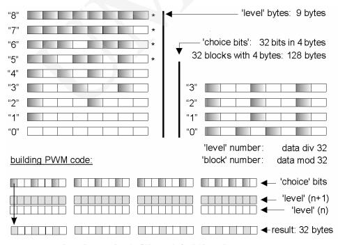
Fig. 6. Constructing the filling code for 8-bit DAC\_PWM converter
