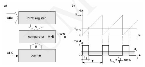
Fig.2. Structure of the PWM signal generator and its operating rule
