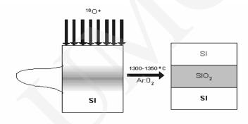
Fig. 1. High temperature implantation in connection with thermal treatment leads to sharp interfaces of  $SiO_2$  layer
